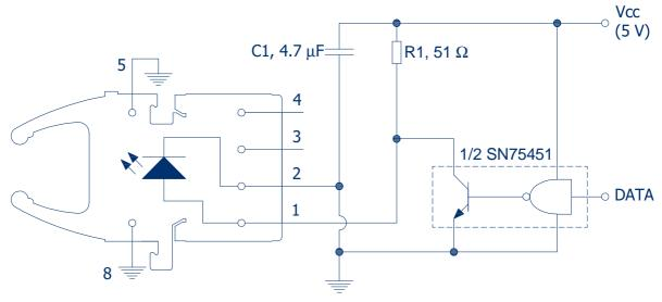
NOTE: R1 = 51  $\Omega$ , then I<sub>F</sub> drive current is approximately 60 mA. To reduce drive current, select a higher R1 value
