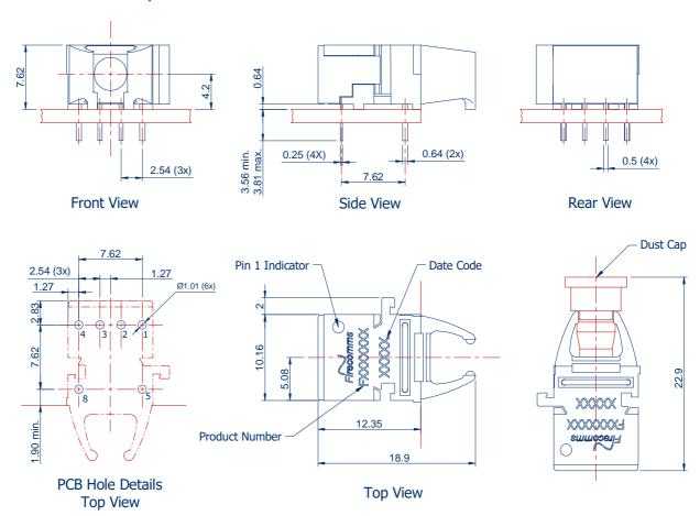
FIGURE 9 Mechanical dimensions of the horizontal connectors and PCB footprint, which is a top view General dimensional tolerance is  $\pm\,0.2~\text{mm}$
